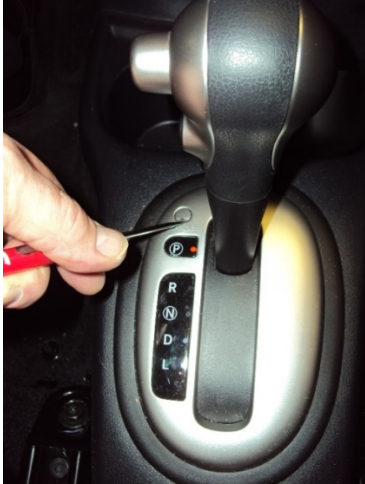
Removing shifter lock cap
